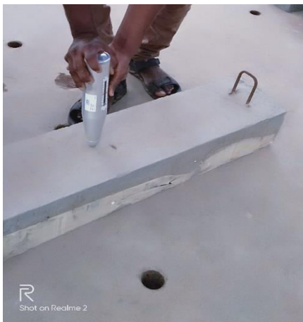
Figure 1. Rebound Hammer Test
